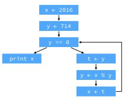
**RTL/CFG** is the name given to intermediate representations where each function of the program is represented as a control-flow graph whose node contain RTL instructions.
