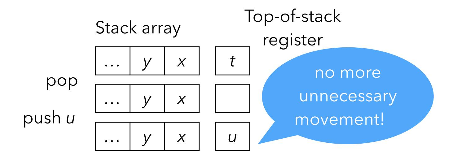
Beware: caching a variable number of stack elements means that every instruction must have one implementation per **cache state** (number of stack elements currently cached)
